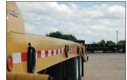
CAMBERED FRAME FOR INCREASED STRENGTH & WEIGHT DISTRIBUTION
